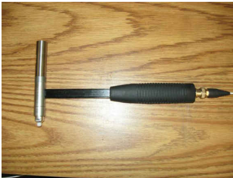
Figure 5-1 PCB Impact Hammer
